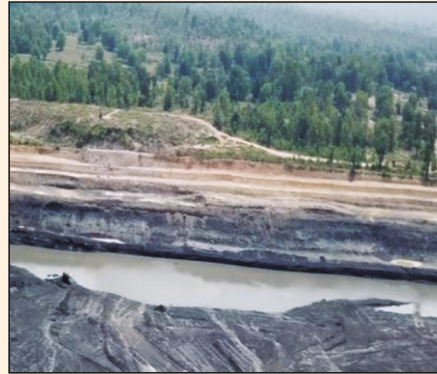
Mine Sump to collect rainwater
